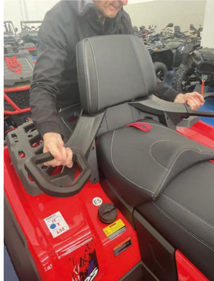
Step 2: Remove the driver's seat, using the lever located in the position indicated in the picture below.
