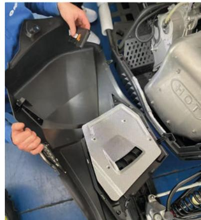
Step 2: Remove the protective cap (circled in red) on the diagnostic port and insert the connector
