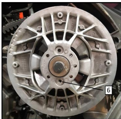
Fig. 33 6. Transformer belt installation
